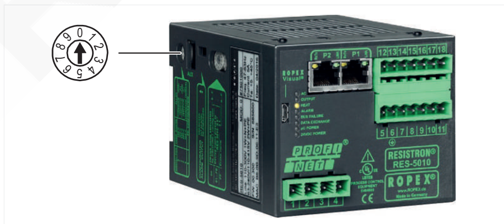
Illustration 7: Position of coding dial for temperature range and alloy
