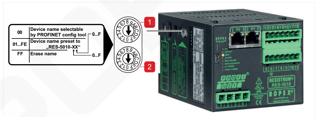
Illustration 8: Position of coding dial for station name
